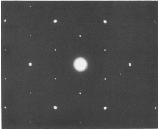
Figure 11 Electron diffraction diagram of sample EA-3 after heat treatment showing monocrystalline hexagonal chalcocite (at 105°C).
