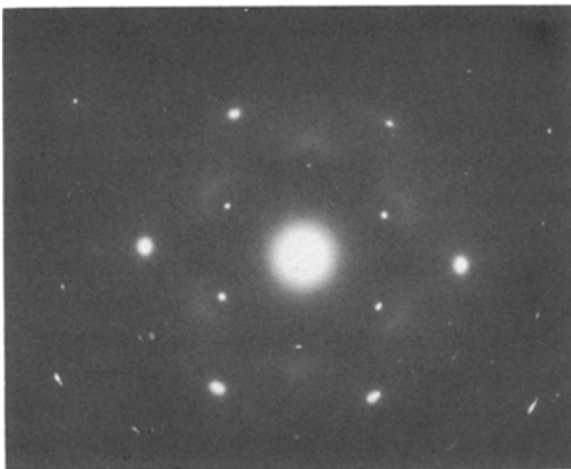
Figure 12 Electron diffraction diagram of the same sample as in Fig. 11, at 85°C, showing hexagonal chalcocite with some haloes.
